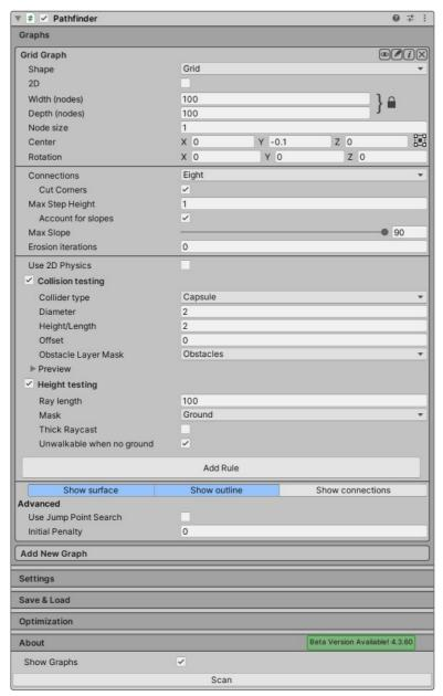
As the name implies, the GridGraph will generate a grid of nodes with the size width\*depth. A grid can be positioned anywhere in the scene, and you can rotate it any way you want.
